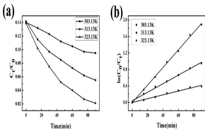
Figure 6. Effect of temperature on the kinetics of phenol degradation in the presence of 0.5 wt% TiO<sub>2</sub>/CDs.
