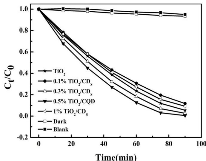
Figure 4. Photocatalytic degradation of phenol in the presence of TiO<sub>2</sub>/CD composites ( $C_0$  and  $C_t$  represent the initial concentration of phenol and that after time  $t$ , respectively).
