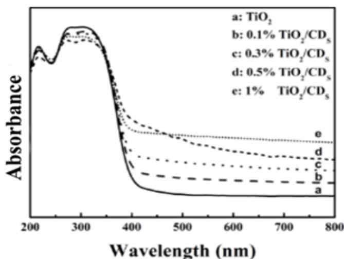
Figure 3. UV-vis diffuse reflectance spectra of TiO<sub>2</sub>/CD nanocomposites.
