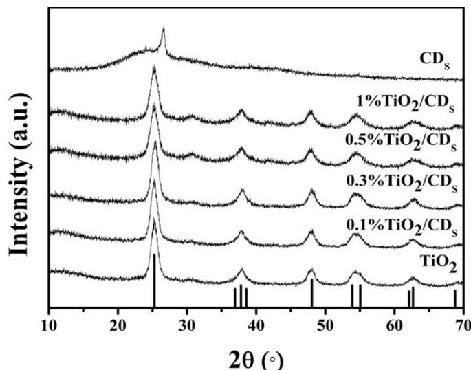
Figure 1: XRD patterns of TiO<sub>2</sub>/CD nanocomposites.
