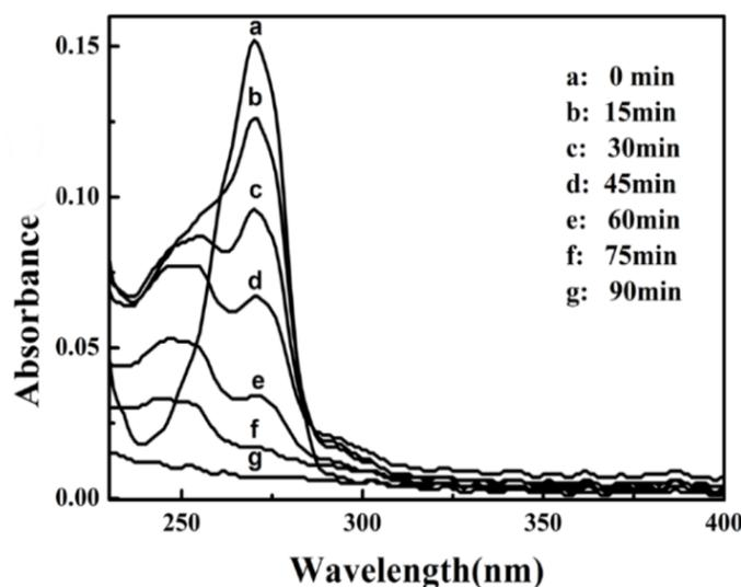
Figure 5. UV-vis absorption spectra of (phenol + 0.5 wt% TiO<sub>2</sub>/CD) systems irradiated for different times.
