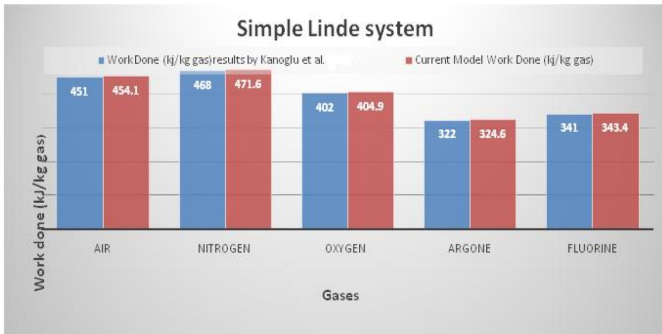
Fig. 1(d) Validation results of work done in current model and literature[7]
