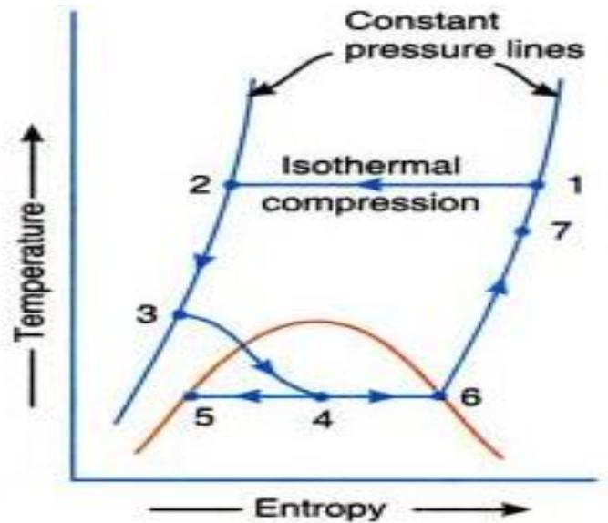
Fig: 1(b) Schematics Linde Hampson System T-S diagram [7]
