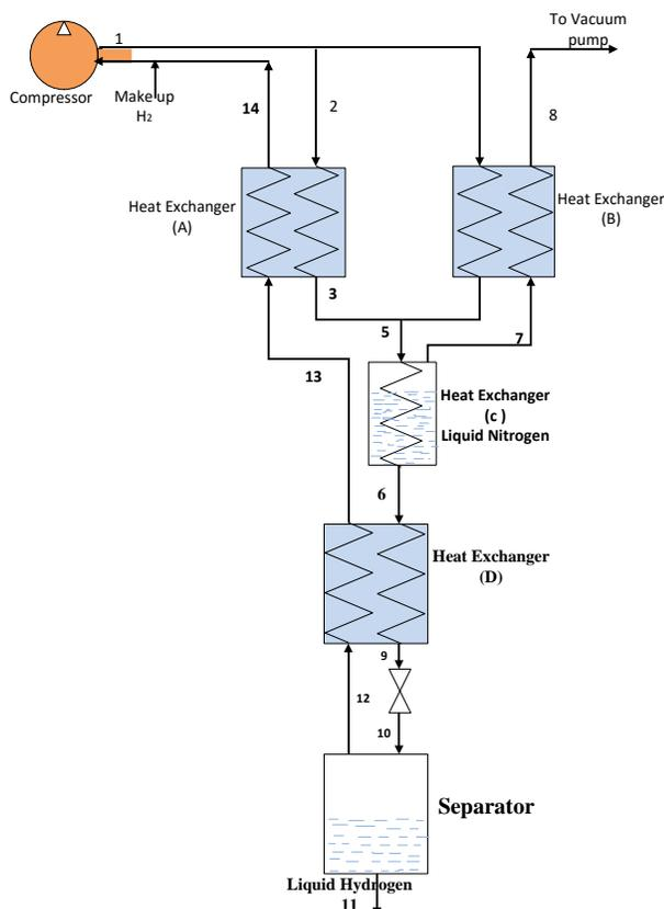
Fig. 5. Block diagram of hydrogen liquefaction system
