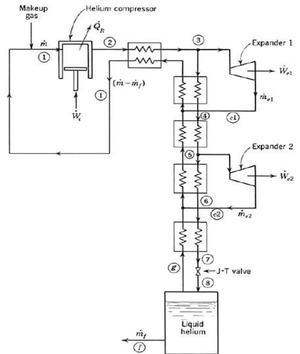
Fig: 6. (a) Schematic of Collin system
