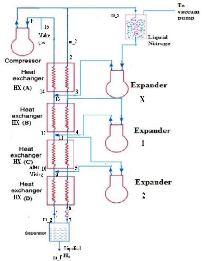
Fig: 8 Block diagram of modified Helium liquefaction system
