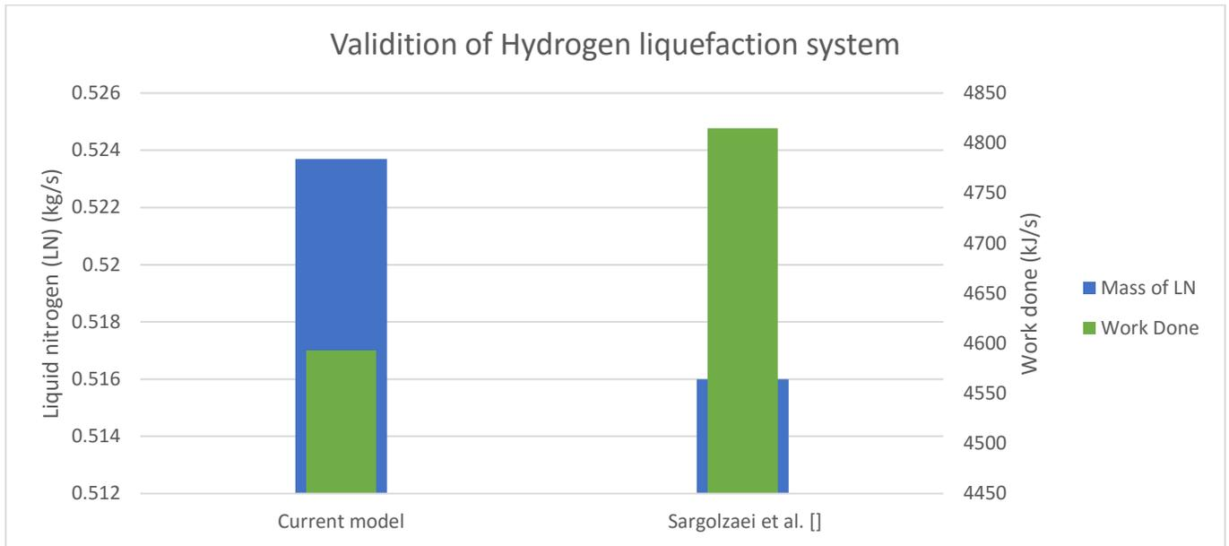
Fig.7 Validation results of liquid nitrogen and work done in current model and literature
