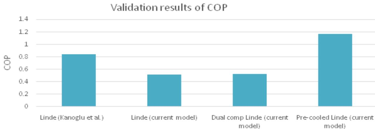
Fig.3. Validation results of COP in current model and literature for different systems
