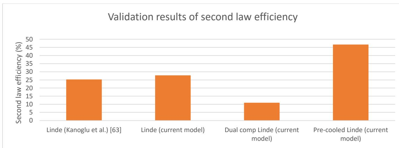
Fig.4: Validation results of second law efficiency in current mode and literature of different Linde, Dual compressor Linde, Pre-cooled Linde system
