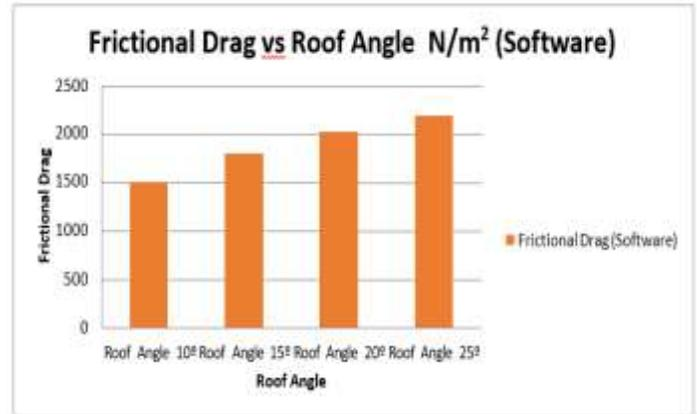
Figure 2: Frictional Drag of different roof angle after software (STAAD-Pro)
