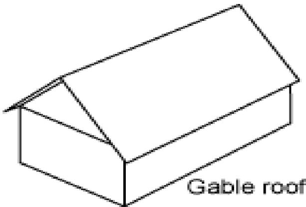
Figure 1: Schematic diagram of Gable roof
