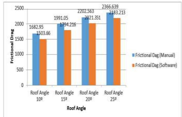
Figure 3: Frictional Drag of different roof angle after manual and software (STAAD-Pro)
