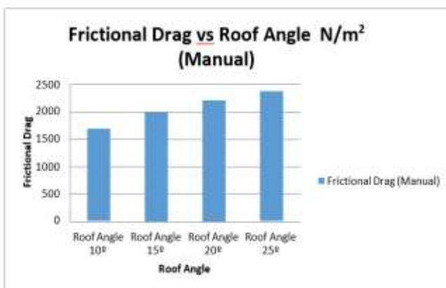
Figure 1: Frictional Drag of different roof angle after manual calculation
