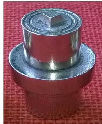
Figure 1: Square pin profiled tool [13]
