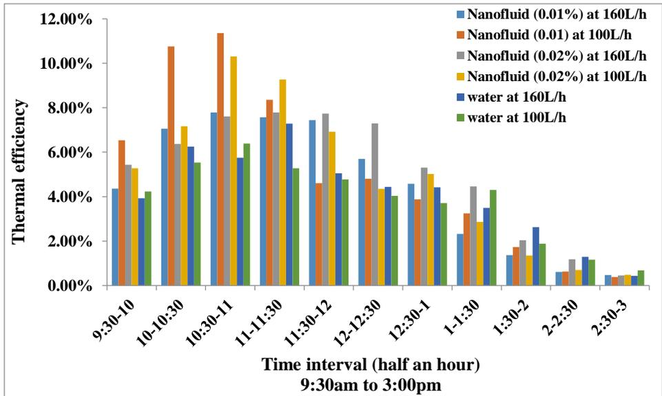
Figure 3: Experimental variations in overall thermal efficiency for different fluids [17]
