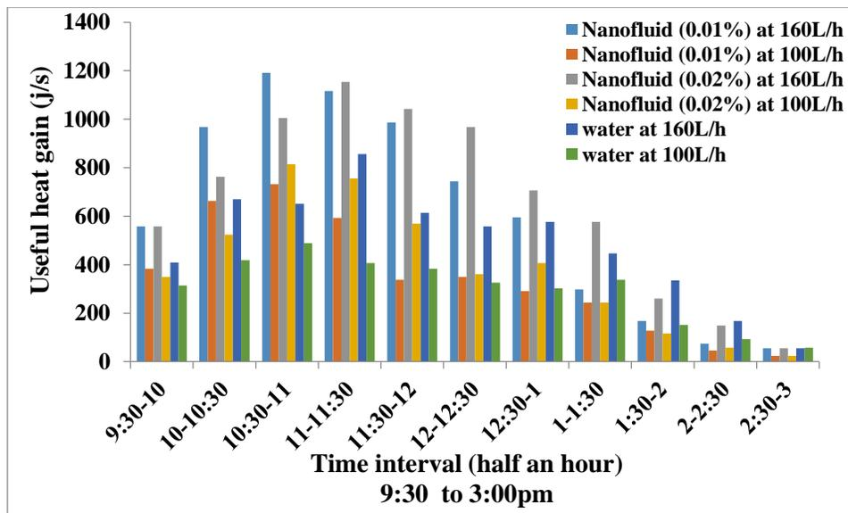
Figure 1: Experimental variation in useful heat gain by nano fluid and water at different conc. and volume flow rates [17]
