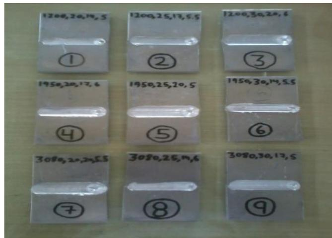
Figure 1: Plate after friction stir welding
