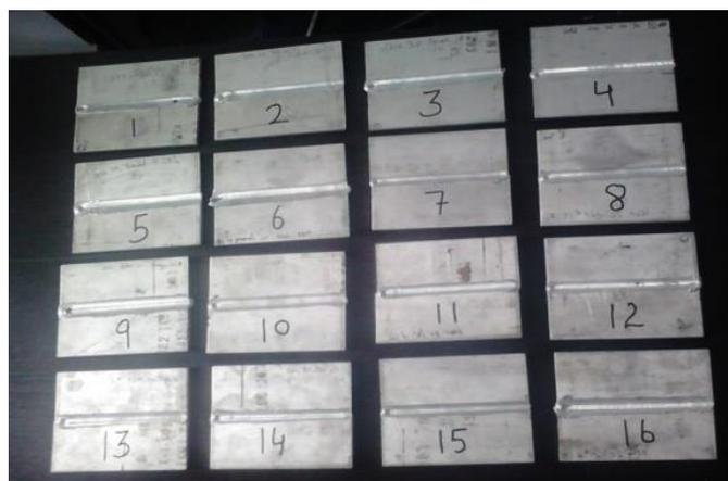
Figure 2: Plate after friction stir welding
