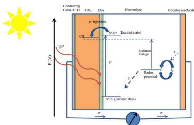
Figure 1: Construction of dye-sensitized nano-crystalline solar cell [16].
