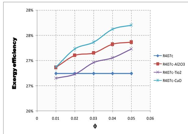
Fig.36. Variation of Exergy Efficiency with volume fraction ( $\phi$ ) of VCRS with R407c using different nanoparticles
