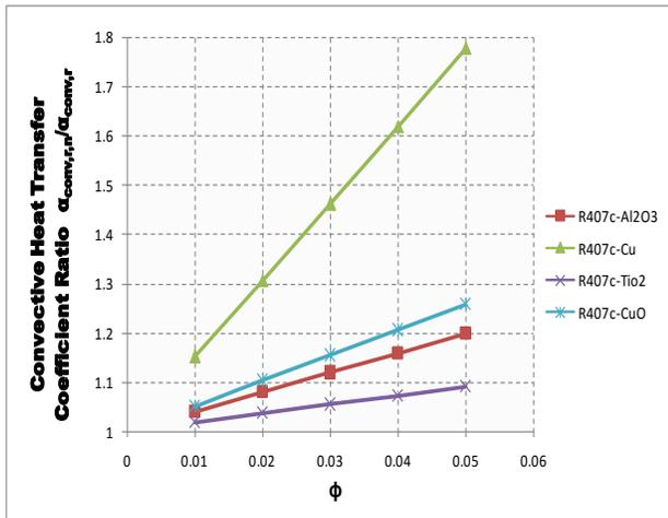
Fig.23. Variation of Convective heat transfer coefficient ratio with volume fraction ( $\phi$ ) of R407c using different nanoparticles
