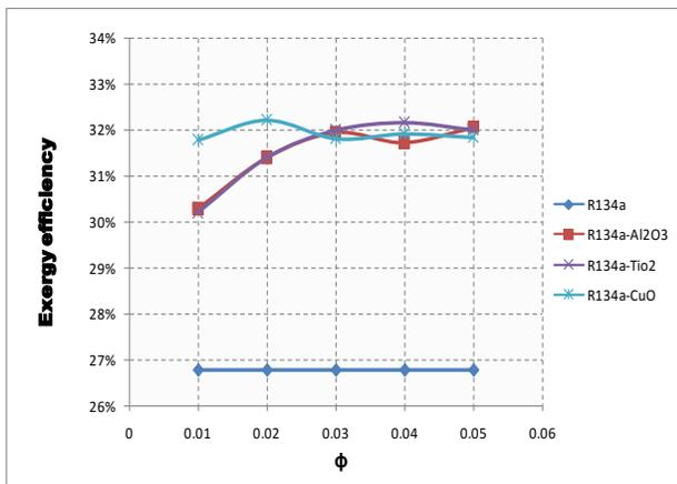
Fig.35 Variation of Exergy Efficiency with volume fraction ( $\phi$ ) of VCRS with R134a using different nanoparticles
