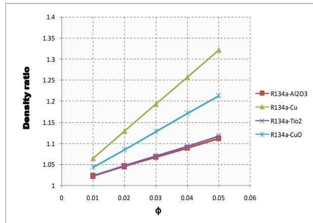
Fig.14 Variation of Density Ratio with volume fraction ( $\phi$ ) of R134a using different nanoparticles
