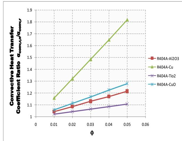
Fig.24 Variation of Convective heat transfer coefficient ratio with volume fraction ( $\phi$ ) of R404A using different nanoparticles
