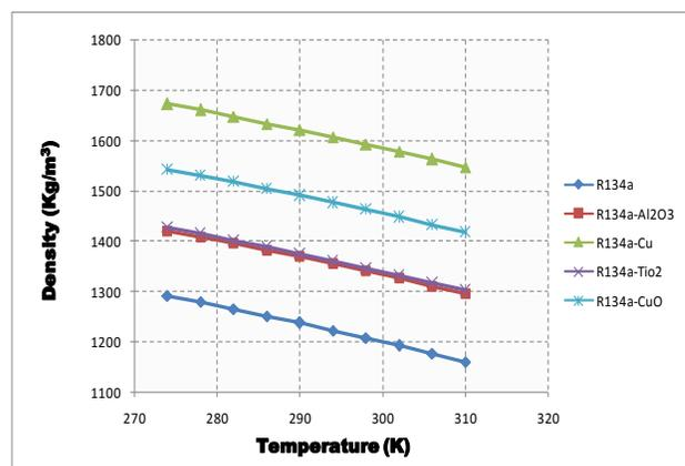
Fig.4 Variation of Density with Temperature of R134a using different nanoparticles
