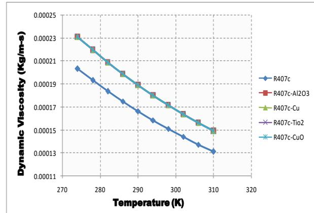
Fig.8 Variation of Dynamic viscosity with Temperature of R407c using different nanoparticles
