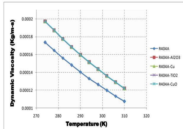
Fig.9: Variation of Dynamic viscosity with Temperature of R404A using different nanoparticles
