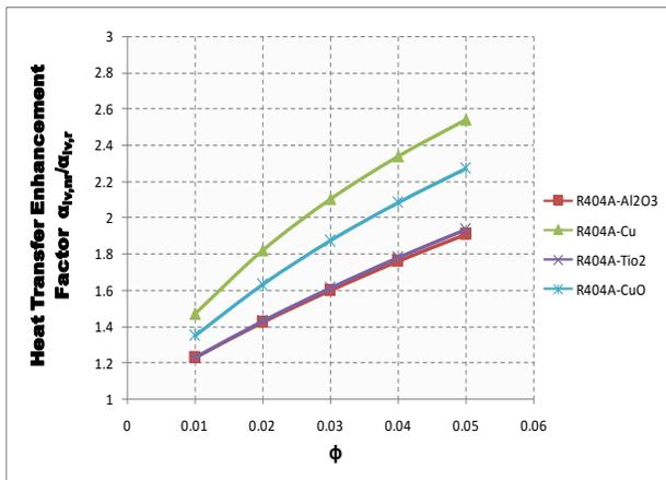
Fig.27 Variation of Heat transfer Enhancement Factor with volume fraction ( $\phi$ ) of R404A using different nanoparticles
