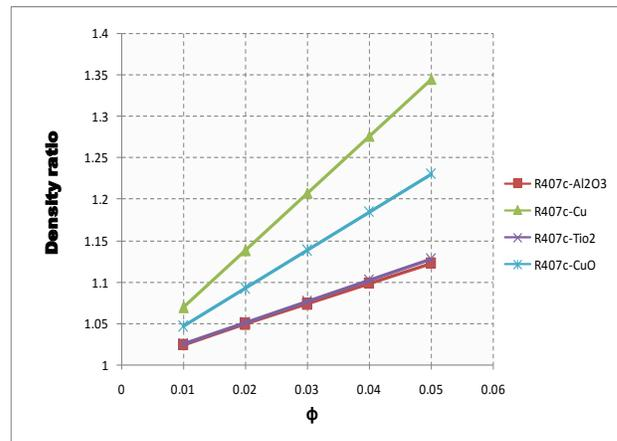
Fig.13 Variation of Density Ratio with volume fraction ( $\phi$ ) of R407c using different nanoparticles
