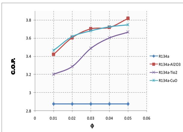
Fig.29 Variation of C.O.P with volume fraction ( $\phi$ ) of VCERS with R134a using different nanoparticles
