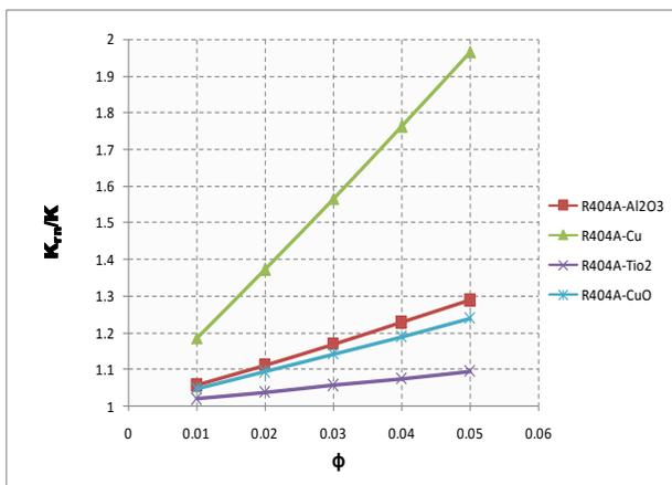
Fig.18 Variation of Thermal conductivity Ratio with volume fraction ( $\phi$ ) of R404A using different nanoparticles
