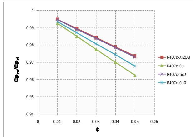
Fig.19 Variation of Specific heat ratio with volume fraction ( $\phi$ ) of R407c using different nanoparticles
