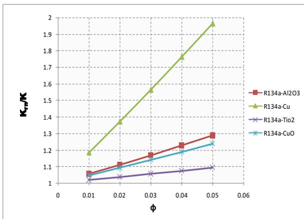
Fig.17 Variation of Thermal conductivity Ratio with volume fraction ( $\phi$ ) of R134a using different nanoparticles
