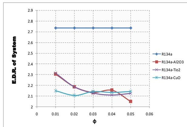
Fig.32 Variation of Exergy destruction ratio with volume fraction ( $\phi$ ) of VCERS with R134a using different nanoparticles
