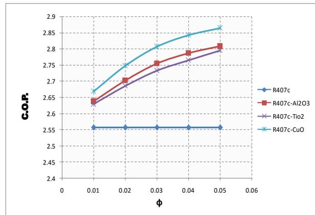
Fig.30 Variation of C.O.P with volume fraction ( $\phi$ ) of VCERS with R407c using different nanoparticles
