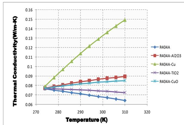
Fig.3. Variation of Thermal conductivity with Temperature of R404A using different nanoparticles
