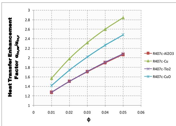
Fig.28 Variation of Heat transfer Enhancement Factor with volume fraction ( $\phi$ ) of R407c using different nanoparticles
