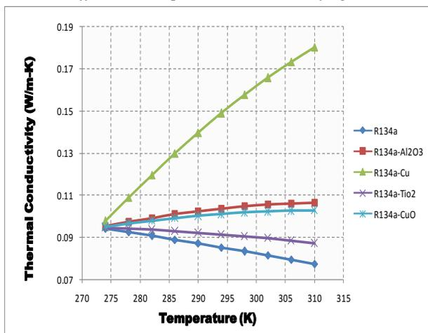
Fig.1: Variation of Thermal conductivity with Temperature of R134a using different nanoparticles
