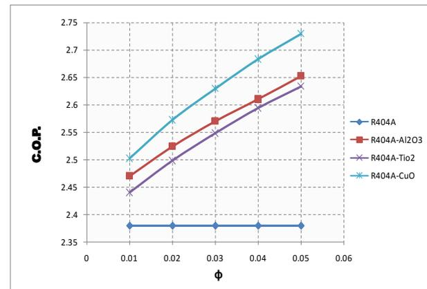
Fig.31: Variation of C.O.P with volume fraction ( $\phi$ ) of VCERS with R404A using different nanoparticles
