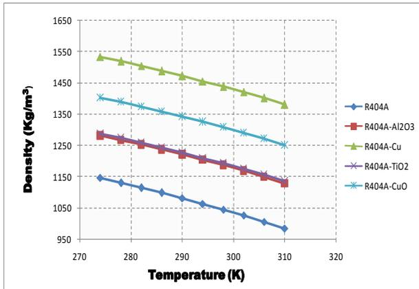
Fig.5 Variation of Density with Temperature of R404A with temperature using different nanoparticles
