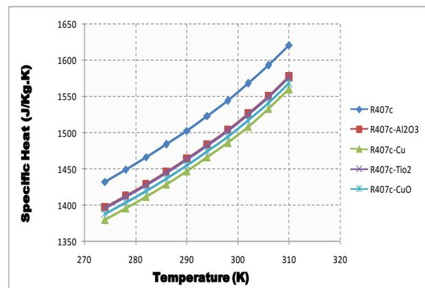
Fig.10 Variation of Specific heat with Temperature of R407c using different nanoparticles
