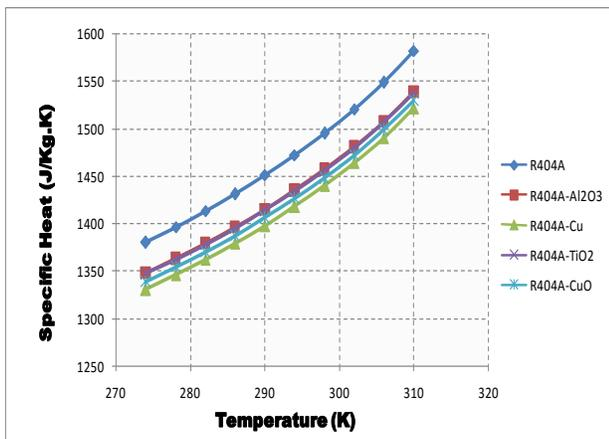
Fig.12 Variation of Specific heat with Temperature of R404A using different nanoparticles
