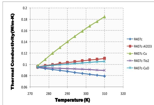
Fig.2; Variation of Thermal conductivity with Temperature of R407c using different nanoparticles
