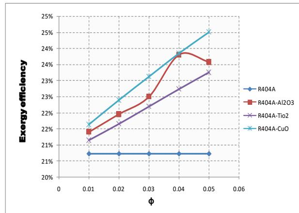
Fig.37 Variation of Exergy Efficiency with volume fraction ( $\phi$ ) of VCRS with R404A using different nanoparticles
