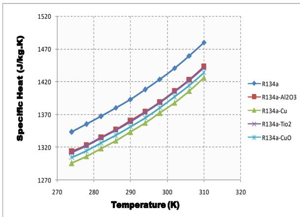
Fig.11 Variation of Specific heat with Temperature of R134a using different nanoparticles
