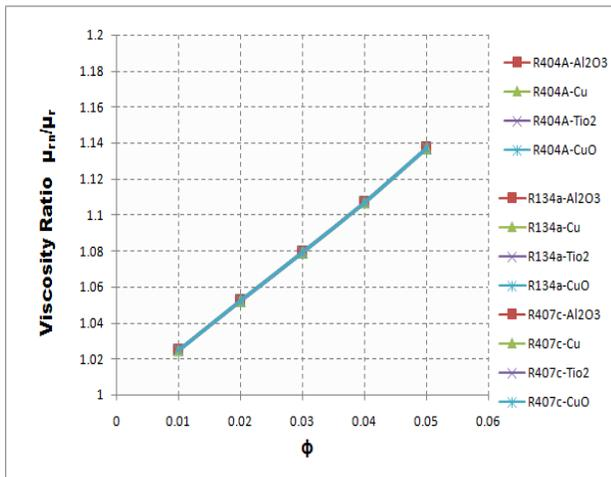
Fig.22 Variation of Viscosity ratio with volume fraction ( $\phi$ ) of all Nano refrigerant
