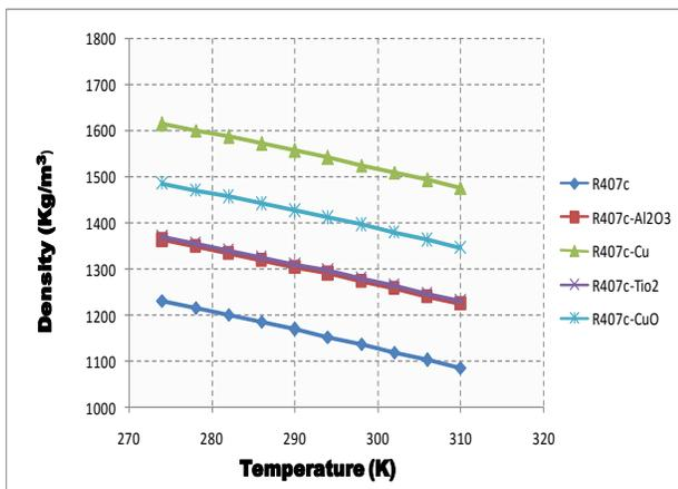
Fig.6 Variation of Density with Temperature of R407c using different nanoparticles
