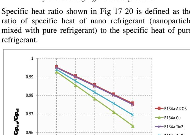
Fig.21 Variation of Specific heat ratio with volume fraction ( $\phi$ ) of R134a using different nanoparticles
