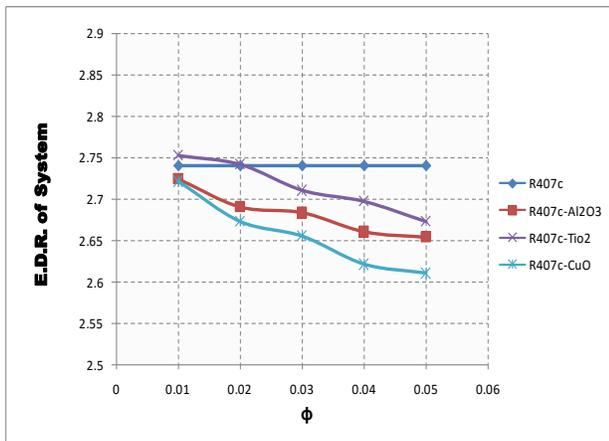
Fig.33 Variation of Exergy Destruction ratio with volume fraction ( $\phi$ ) of VCRS with R407c using different nanoparticles
