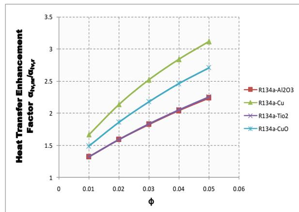
Fig.26. Variation of Heat transfer Enhancement Factor with volume fraction ( $\phi$ ) of R134a using different nanoparticles
