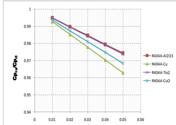
Fig.20: Variation of Specific heat ratio with volume fraction ( $\phi$ ) of R404A using different nanoparticles
