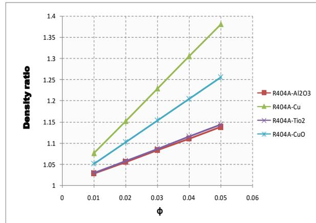
Fig.15. Variation of Density Ratio with volume fraction ( $\phi$ ) of R404A using different nanoparticles
