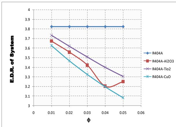
Fig.34 Variation of Exergy destruction ratio with volume fraction ( $\phi$ ) of VCRS with R404A using different nanoparticles
