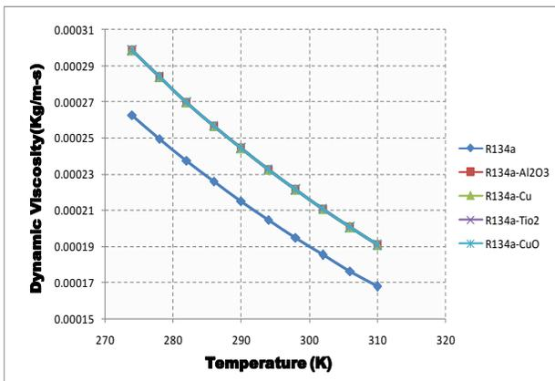
Fig.7 Variation of Dynamic viscosity with Temperature of R134a using different nanoparticles
