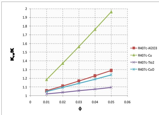
Fig.16 Variation of Thermal conductivity Ratio with volume fraction ( $\phi$ ) of R407c using different nanoparticles
