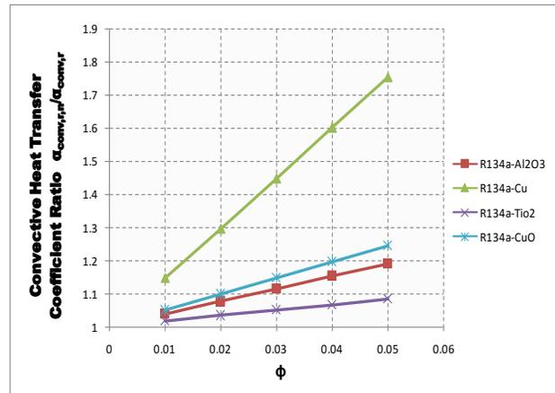
Fig.25. Variation of Convective heat transfer coefficient ratio with volume fraction ( $\phi$ ) of R134a using different nanoparticles
