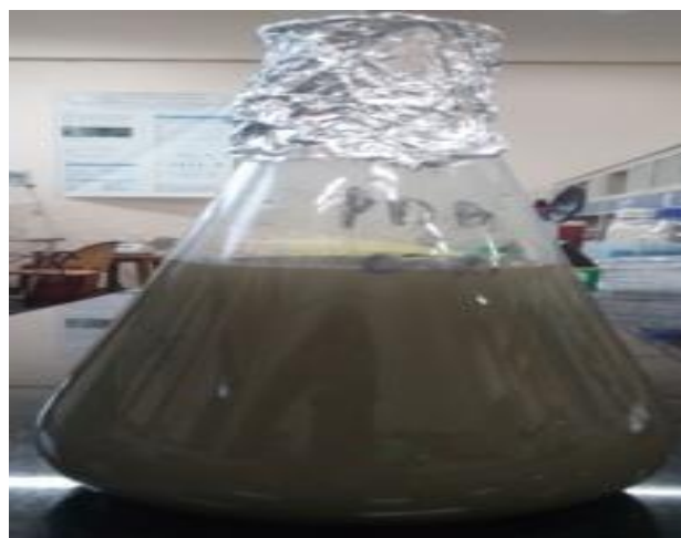
Figure: 13 Nano particle settlement after 14 hours
