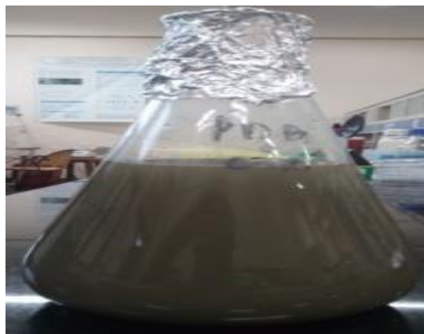
Figure: 11 Nano particle settlement after 10 hours
