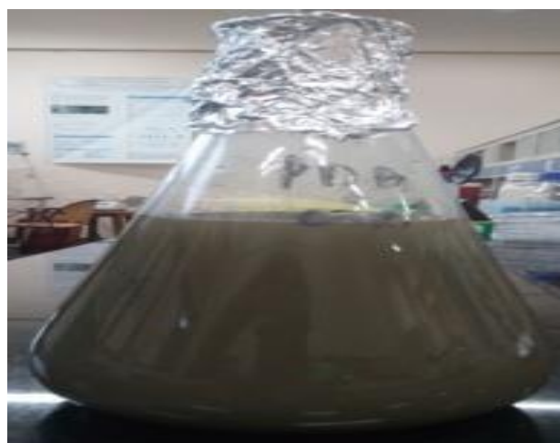
Figure: 12 Nano particle settlement after 12 hours
