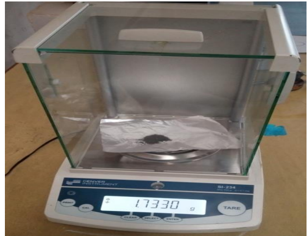
Figure: 5 volume concentration ratio silver nanoparticles were measured by digital balance
