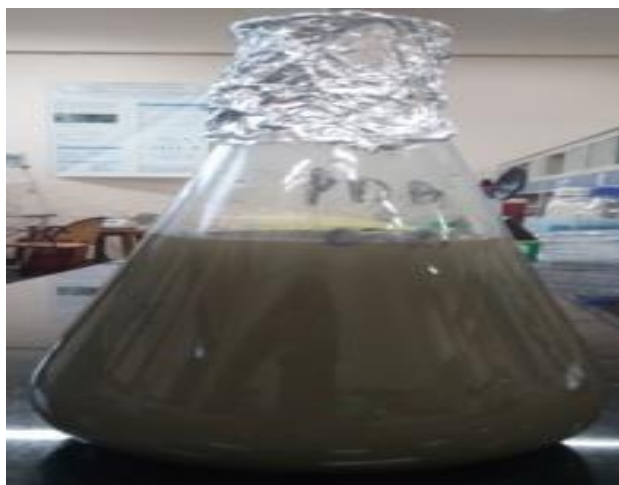
Figure: 8 Nano particle settlement after 4 hours
