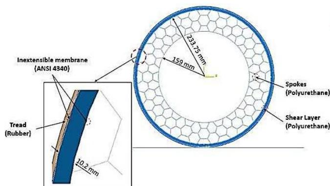
Figure 1: Different parts and dimensions of NPT [12].
