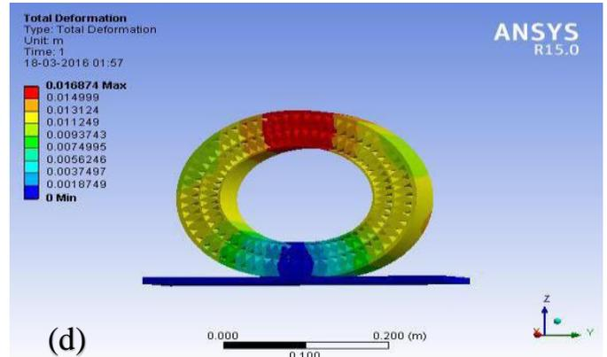
Figure 4: Deflection of air less tyre, (a) Honey Comb Structure, (b) Spoke type Structure, (c) Triangular type Structure, (d) h diamond Structure [15]
