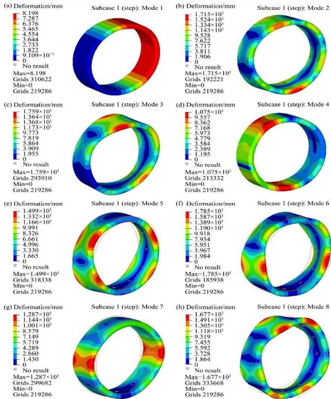
Figure 3: Wheel vibration modes of first-order to eighth-order with ground constraints [14]
