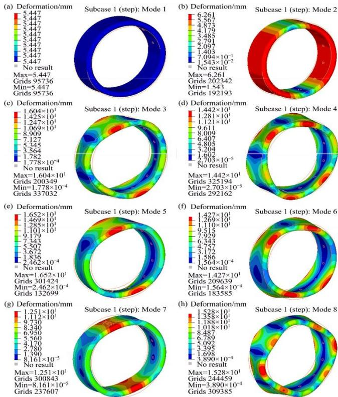
Figure 2: Wheel vibration modes of first-order to eighth-order without ground constraints [14]
