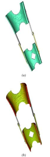
Figure 4 (a) 3D Model of Braces Integrated with connecting structure (b) Wall thickness analysis of braces integrated with connecting structure
