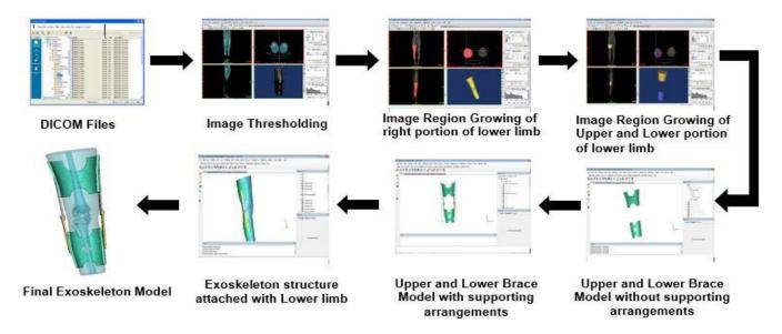
Figure 3. Design sequence of knee exoskeleton
