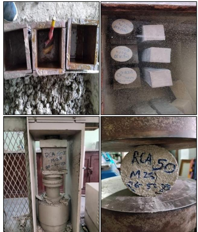
Figure 2: Specimens preparations and experimental testing.
