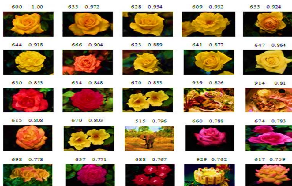
Figure 2(a). The CBIR technique produces a blend of features related to color and shape: Of the top 25, there are 21 images that are similar.
