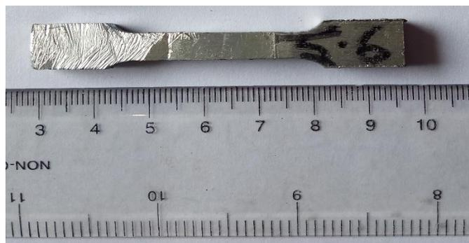
Figure 1: Dimension of tensile test specimen
