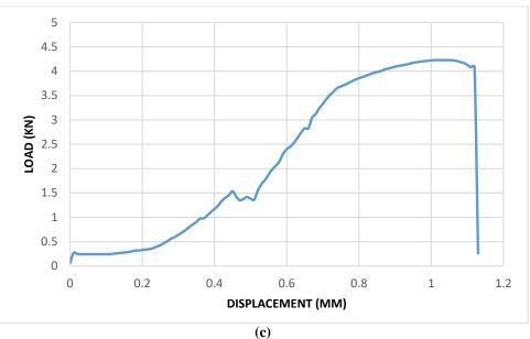
Figure 12: Variation of load displacement of Al-2029 before friction Stir Welding, (a) Specimen-1, (b) Specimen-2, (c) Specimen-3
