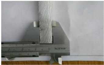
Figure 7: Dimension inspection by Vernier calliper
