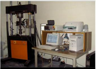
Figure 9: Setup of tensile testing
