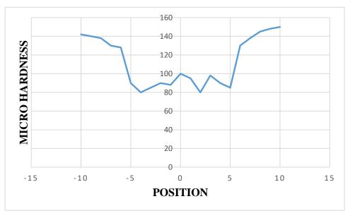
Figure 14: Variation between micro hardness and position
