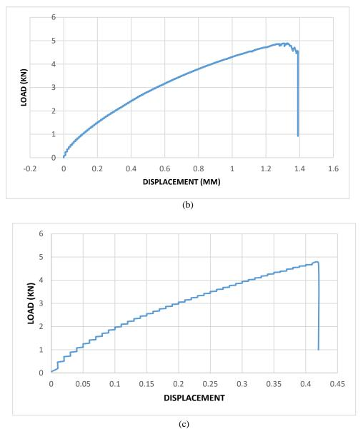
Figure 13: Variation of load displacement of Al-2029 after friction Stir Welding, (a) Specimen-1, (b) Specimen-2, (c) Specimen-3
