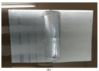
Figure 4: Al-2029 plates before FSW, (b) Al-2029 plates after welding by FSW process
