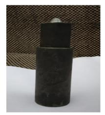
Figure 2: Tool of mild steel for FSW
