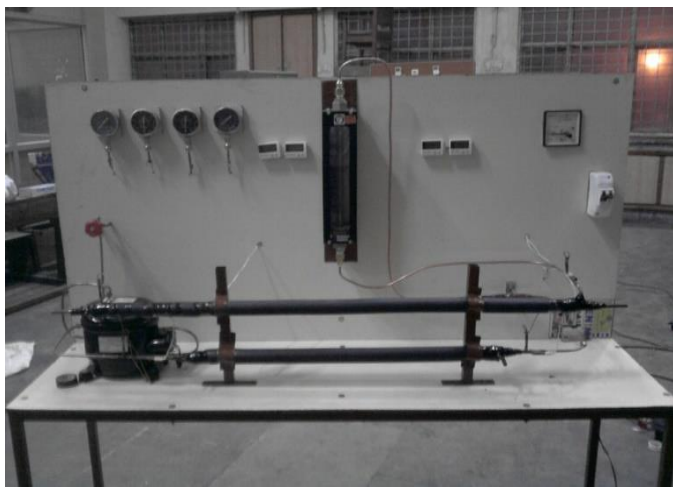
Fig-1(b): Experimental set of variable-speed vapour compression refrigeration systems[39]
