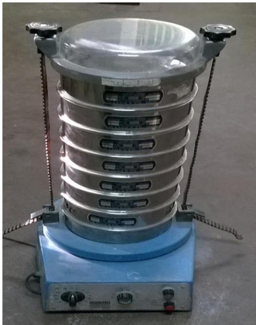
Figure 5. Apparatus setup for sieve analysis
