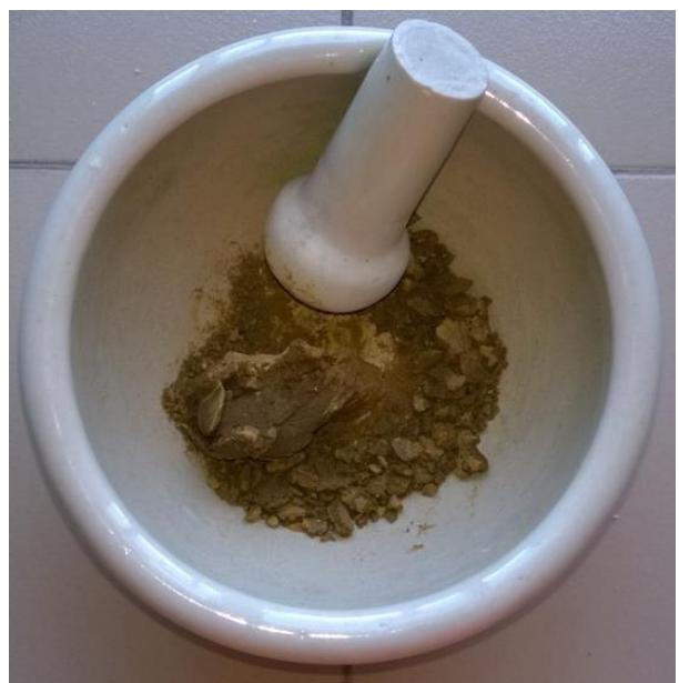
Figure 3. Crushing of dried clay samples
