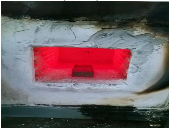
Figure 8. Firing of bricks using a muffle furnace
