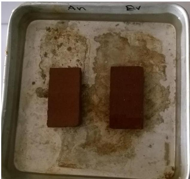
Figure 13. Immersion of bricks in water
