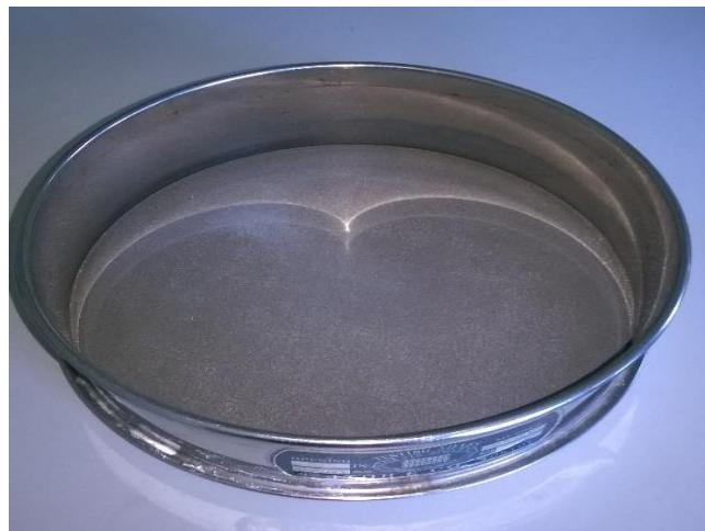
Figure 6. Sieve of 0.075mm
