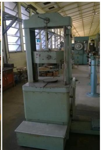
Figure 10. Universal tensile strength testing machine
