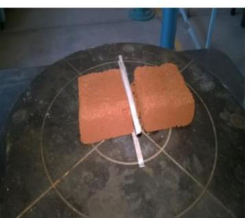
Figure 12. Measuring of splitting tensile load of bricks
