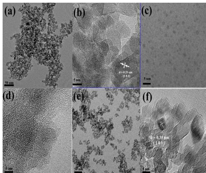
Figure 2. (a, c, e) low- and (b, d, f) high-magnification TEM images of (a, b) pure TiO<sub>2</sub> nanoparticles, (c, d) pure CDs, and (e, f) 0.5 wt% TiO<sub>2</sub>/CDs.
