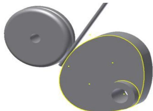
Figure 10: Cam and roller system
