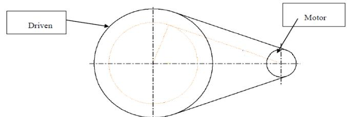
Figure 4: Belt-Pulley free body diagram
