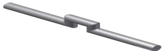
Figure 5: Crankshaft
