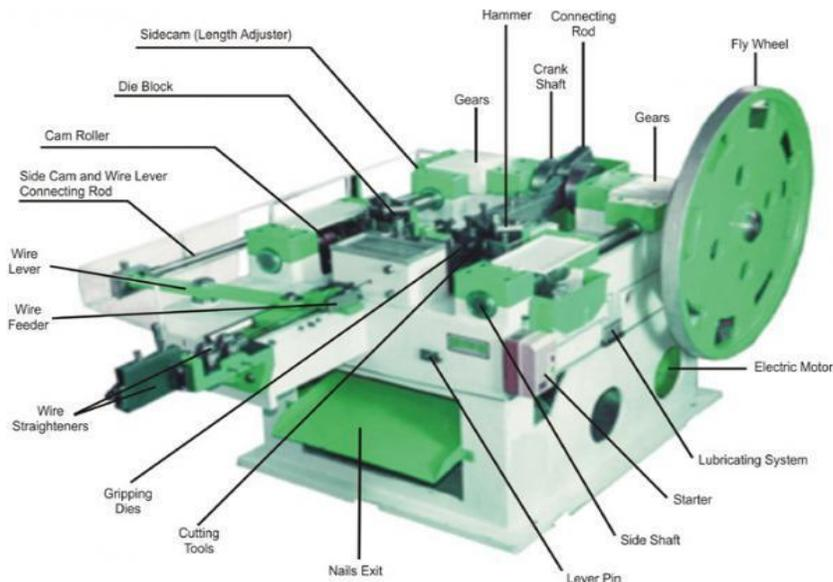
Figure 1: Model of Nail making machine from Punjab, India
