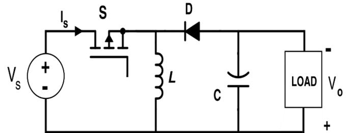
Figure 4: Buck-Boost Converter [6]
