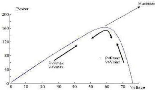
Figure 5: Output power using P&O algorithm [7]
