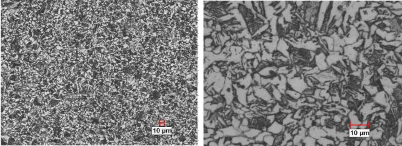
Figure 2: Typical Micro Structure of Dual-phase metal
