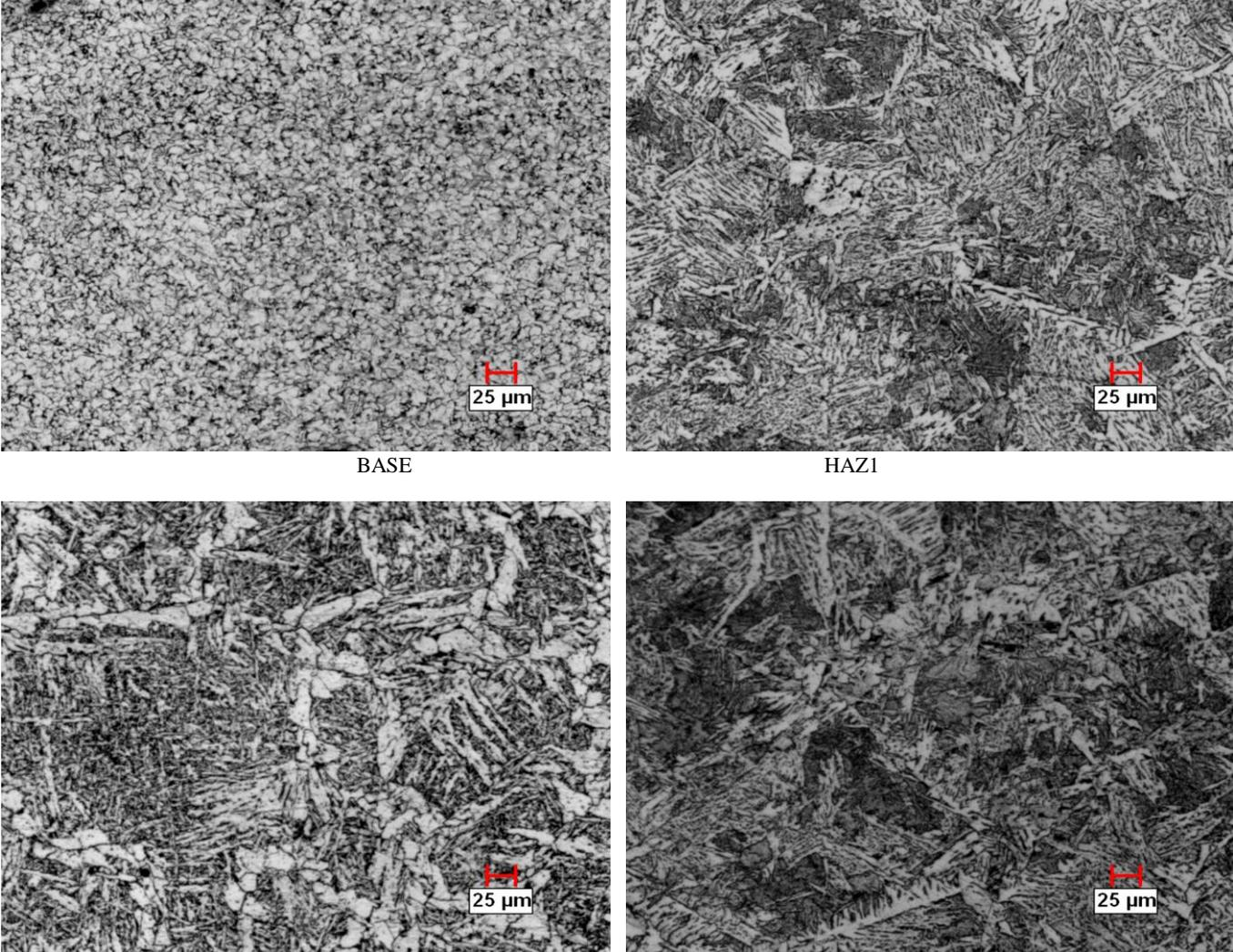
Figure 3: A typical microstructure gradient of weld metal-HAZ-Base metal.
