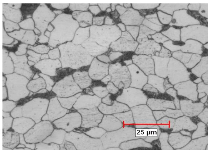
Figure 1: Typical Micro Structure of Base metal
